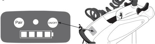
• The four lower LEDs indicate battery condition. They register as green or unlit, depending on charge remaining.
